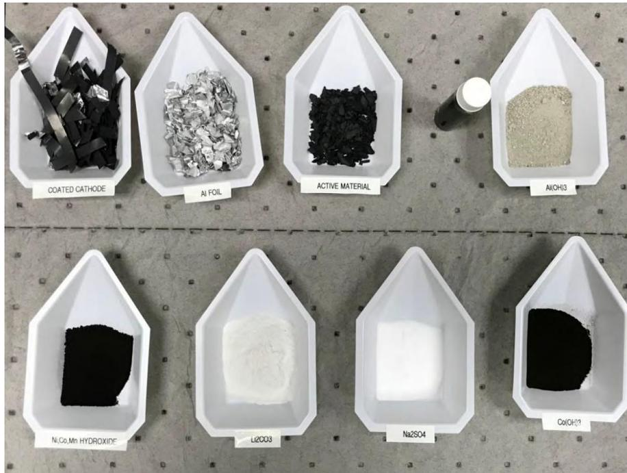
**Figure 24 Outputs from American Manganese EV Battery Recycling Process**
