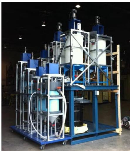
**Figure 22 American Manganese Electrolytic Manganese Dioxide Recovery Pilot Plant (by Kemetco) for Low-Grade Manganese Ores**
