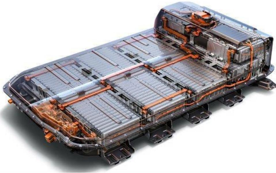
**Figure 56 Chevrolet Bolt Battery Pack<sup>317</sup>**
